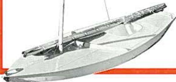
**MAST** and booms are made of special strength anodized aluminum. STARFISH sailboats have actually been sailed in winds that were gusting to 50 mph with no failure or damage to any part of the spars, rigging, hull or sail.
