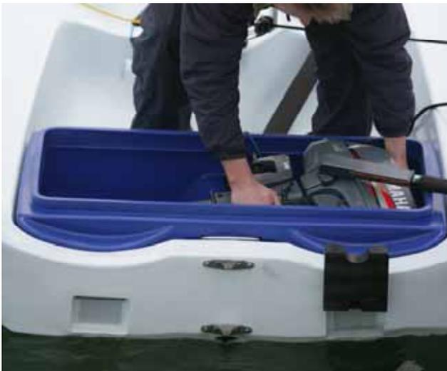
**The storage box is secured in by two eye bolts, one in both sides. Care must be taken when screwing in the eye bolts to avoid cross threading.**
