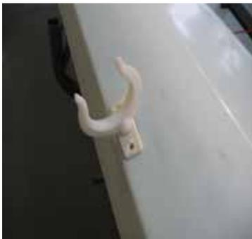
The rowlocks are a push and twist fit into the holes in the gunwhale sides. These can be stored when not in use in the centre console hatch.
