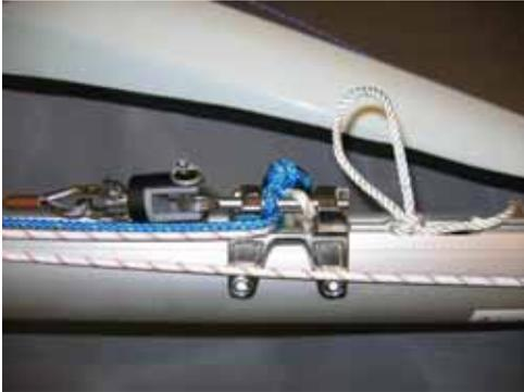
2. Ensure all the halyards are led to the base of the mast and each halyard rope end has a knot tied in it.
