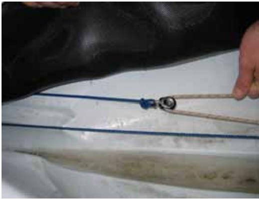
7. Fed the Gennaker halyard through the pole "out" block under the sock.
