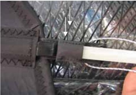
b. To re-tension the batten locate the tip of the prodder in to the location point at the end of the velcro strip then insert between the batten and the batten pocket inner side. Push the prodder until the desired batten tension is attained then withdraw the prodder gently while pressing both sides of the batten pocket together to re-engage the velcro locking mechanism.
