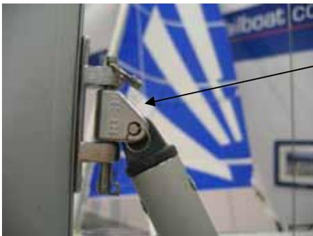
4. Attach the gnav strut to the gnav anchor point using the drop nose pin. (Articulating toggle at the bottom with joint orientation as shown)
