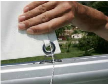
2. Feed the plastic slug slide on the clew outhaul into the cut out on the top of the boom.
