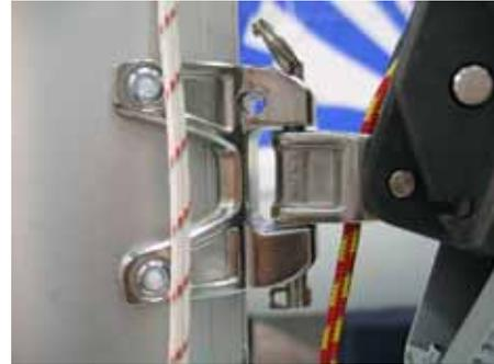
3. Tie the Gnav control line from the boom to the double block and becket at the base of the mast in the boat.
