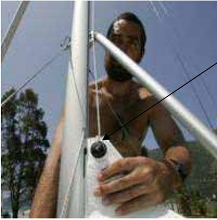
6. Locate the head of the mainsail into the mast track. The GNAV bar must be on the starboard side of the sail with sail and halyard to the port side of the GNAV bar.
