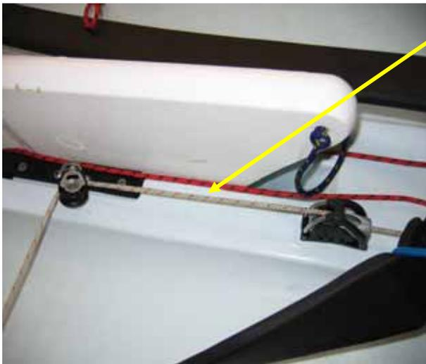
8. Feed the Gennaker halyard through the cleat on the starboard side of the centreboard case and then through the turning block. ( white rope shown)
