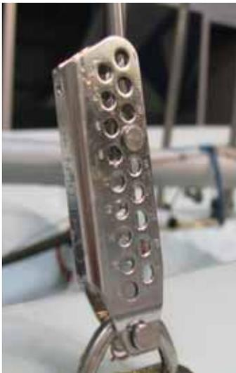
9. Attach the shrouds to the shroud anchor point with the adjuster pin position in the 4th hole down on the back of the vernier adjuster. No 7 engraved on the adjuster.
