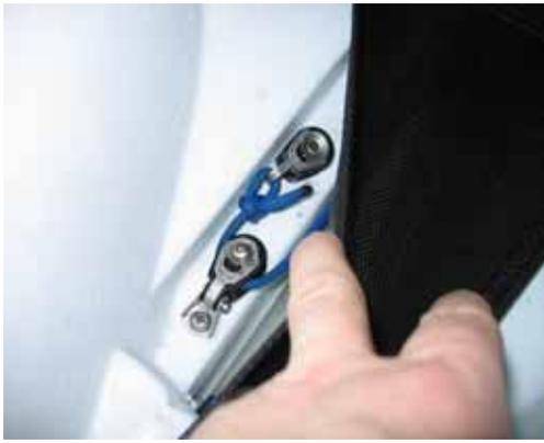
4. Locate the Gennaker pole "out" rope under the Gennaker sock at the bow. This is a blue rope with a block on the end as shown.
