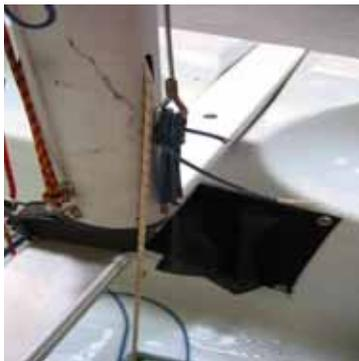
9. Remove the forestay from the jib tack bar and tie to the P clip at the bottom of the mast.
