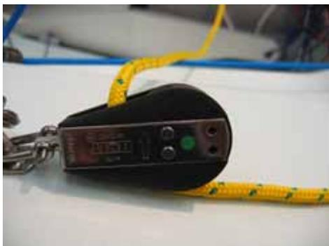
15. Pass the free ends of the gennaker sheets aft (One sheet either side of the jib luff) and through the gennaker sheet ratchet blocks attached to the anchor points. There are arrows on the ratchet block to indicate which way the rope should pass. When under load, the ratchet will engage. (Note – The sheets must pass outside of the shrouds and trapeze lines at all times.)
